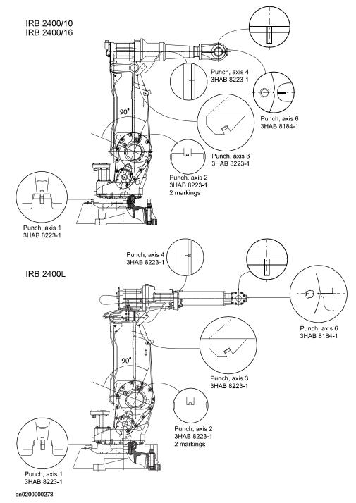
5.4 Calibration movement directions for all axes
